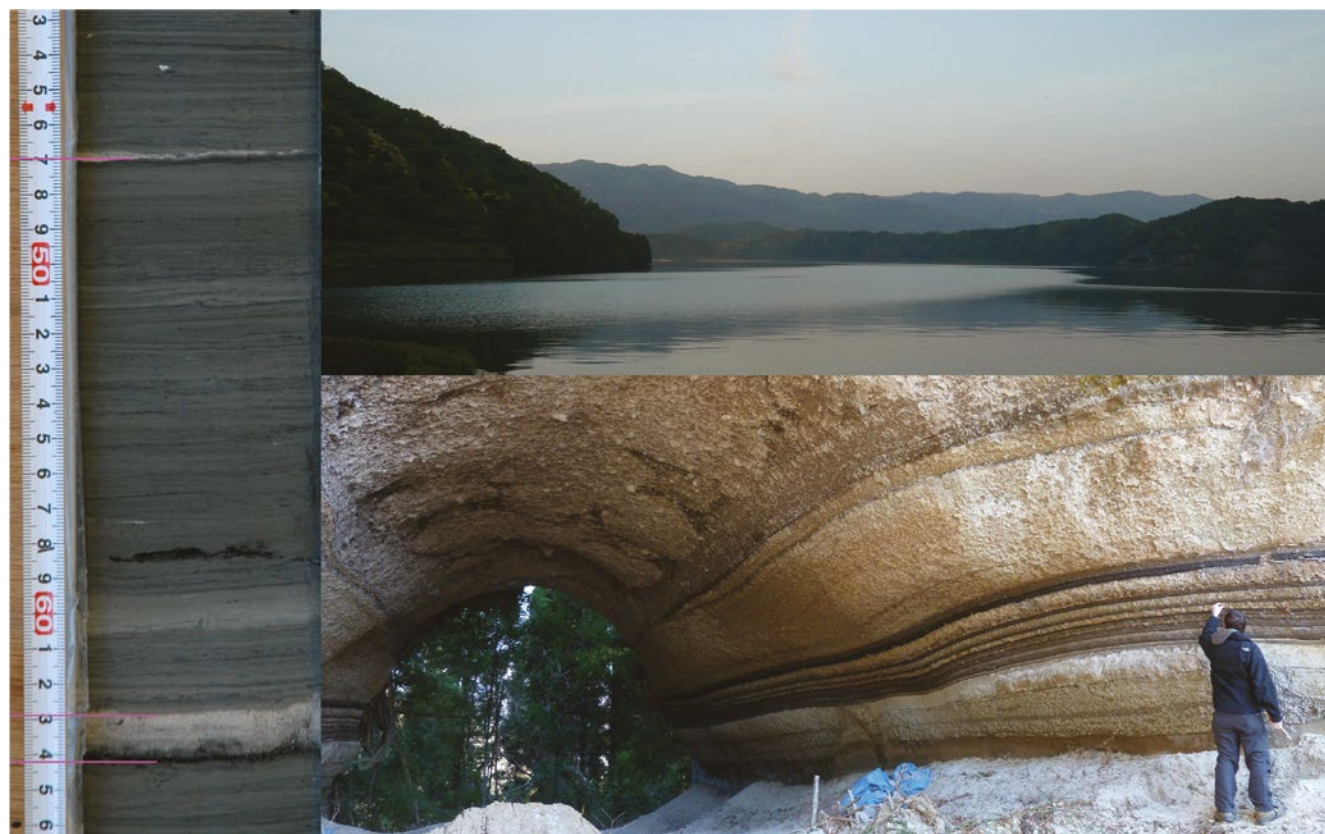
Top right is a photograph of Lake Suigetsu, Japan and left is a section of sediment core extracted. The volcanic ash (tephra) layers are marked. Bottom right is a photograph of a sequence of volcanic deposits in southern Kyushu, Japan. These are the proximal eruption deposits that have been correlated to particular layers in the Lake Suigetsu sediment core using chemistry of the glass shards.
